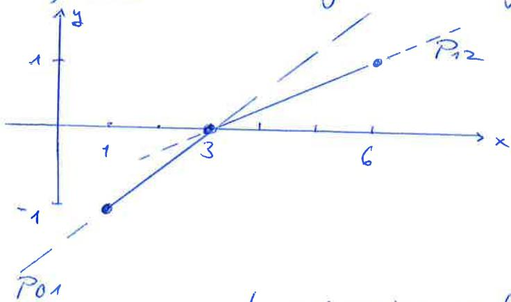
Finally,  $P_{012} = \frac{-(x-x_2)P_{01} + (x-x_0)P_{12}}{x_2 - x_0} = \frac{-(x-6)\left(\frac{x-3}{2}\right) + (x-1)\left(\frac{x-3}{3}\right)}{5}$  (parabola)
